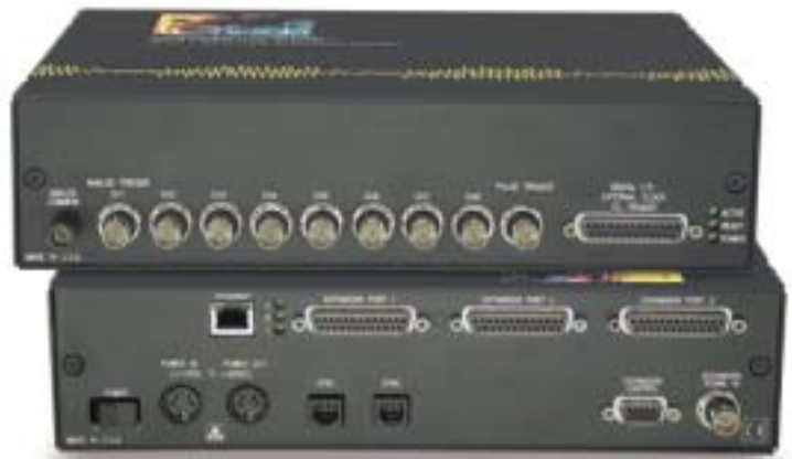
The WaveBook/516E includes a 10/100BaseT Ethernet interface
